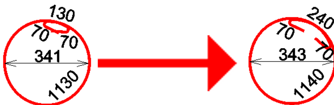
Fig. Circular stirrup before and after overlap change.
